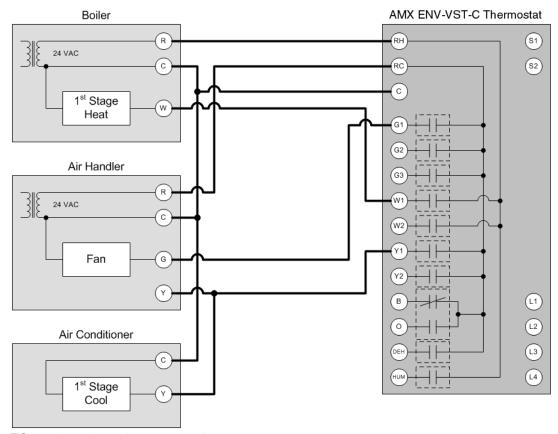
FIG. 7 Boiler and A/C with Separate Transformers wiring
